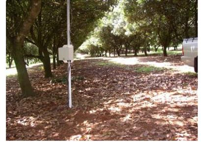
This site presented a difficulty in that GPRS and Next G mobile services were not available where we deployed the soil probes. We developed localised telemetry to transmit soil probe information to a point on the property with mobile phone coverage. From this point we used a repeater device to upload this information to the Peak Environmental Monitoring computer server over the GSM network.
